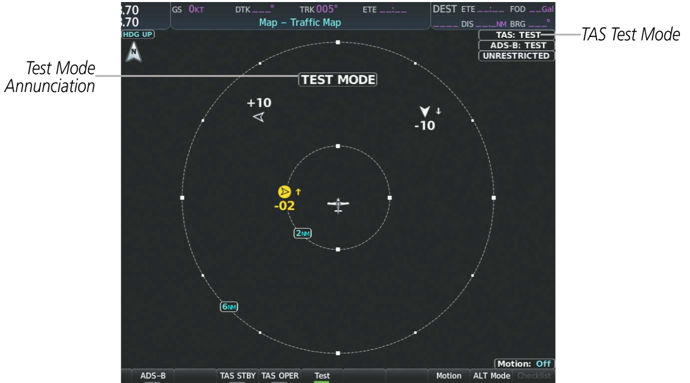
Figure 6-75 System Test in Progress with Test Pattern
