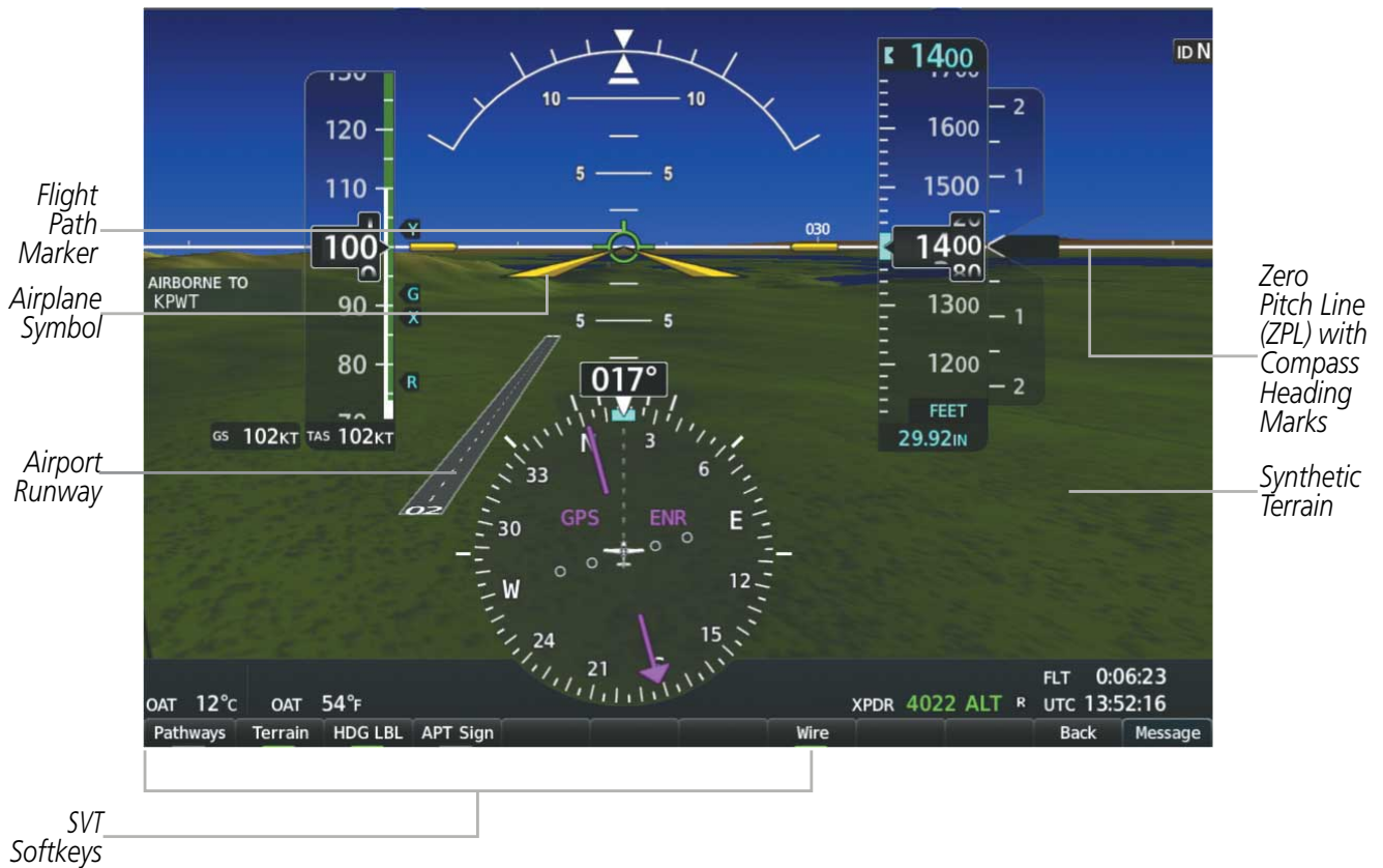
Figure 2-37 SVT on the Primary Flight Display
