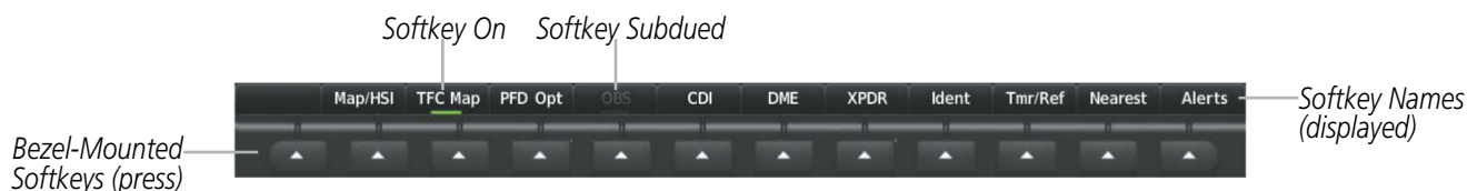
Figure 1-9 Softkeys (First-Level PFD Configuration)
