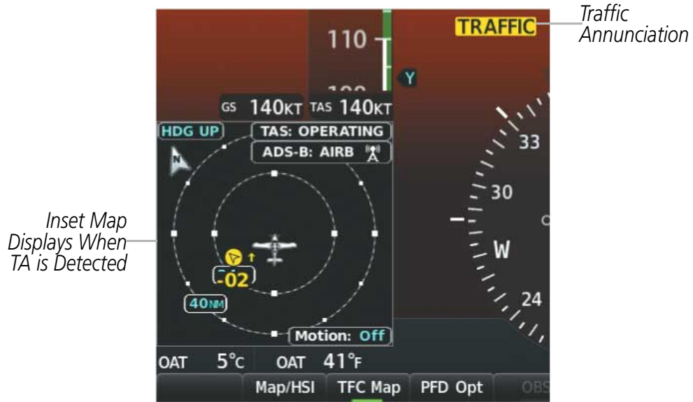
Figure 6-73 Traffic Annunciation on the PFD with Inset Traffic Map
