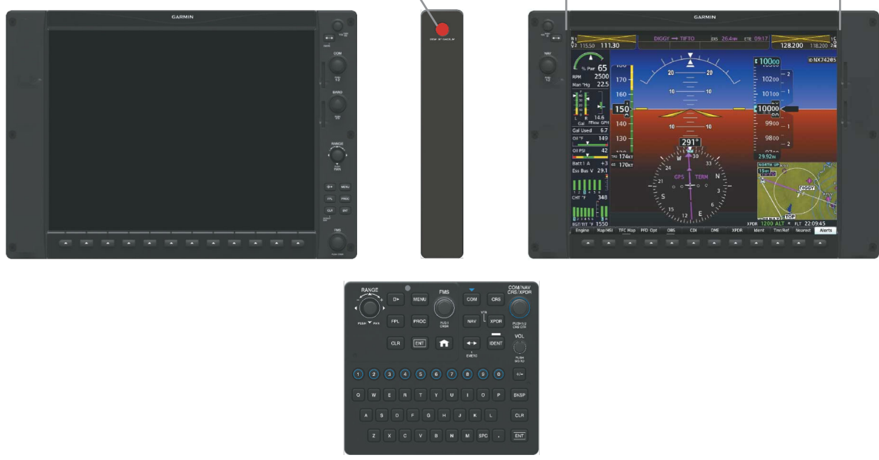
Figure 1-6 Reversionary Mode (Failed PFD)
